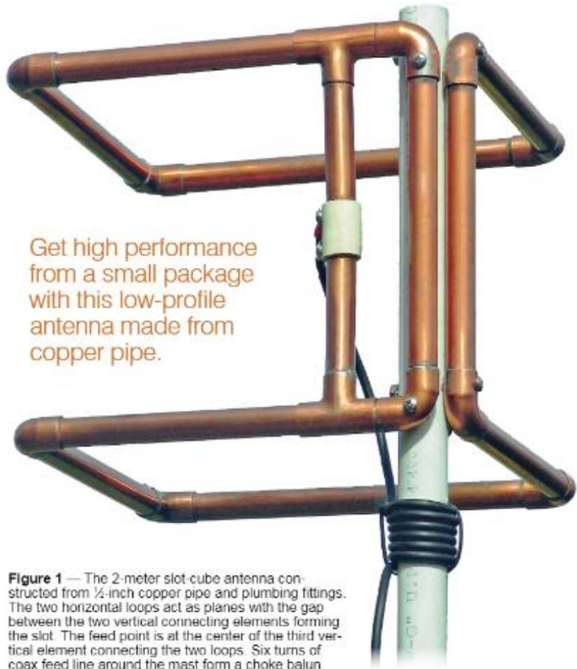
Get high performance from a small package with this low-profile antenna made from copper pipe.
